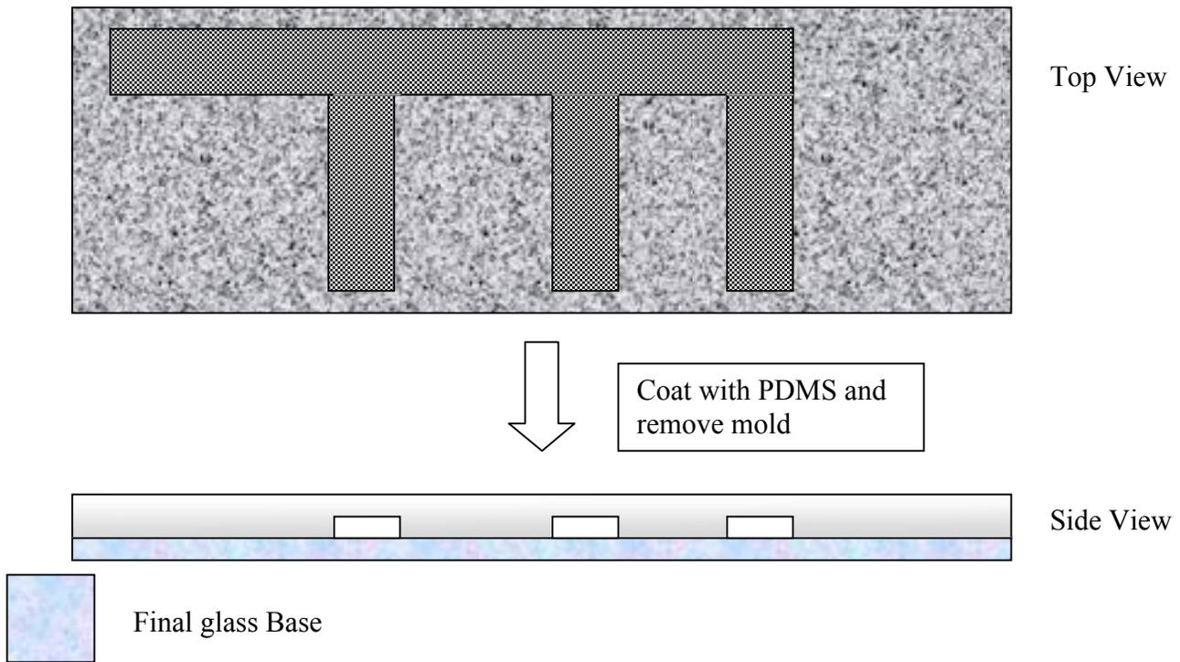
**Figure 4. Coating with PDMS to produce the final chip.**
