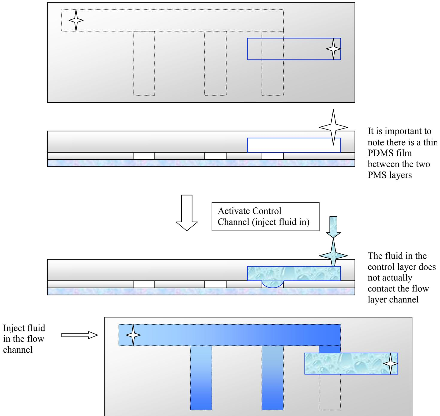
**Figure 6. Action of the control layer on a microfluidic chip.**
