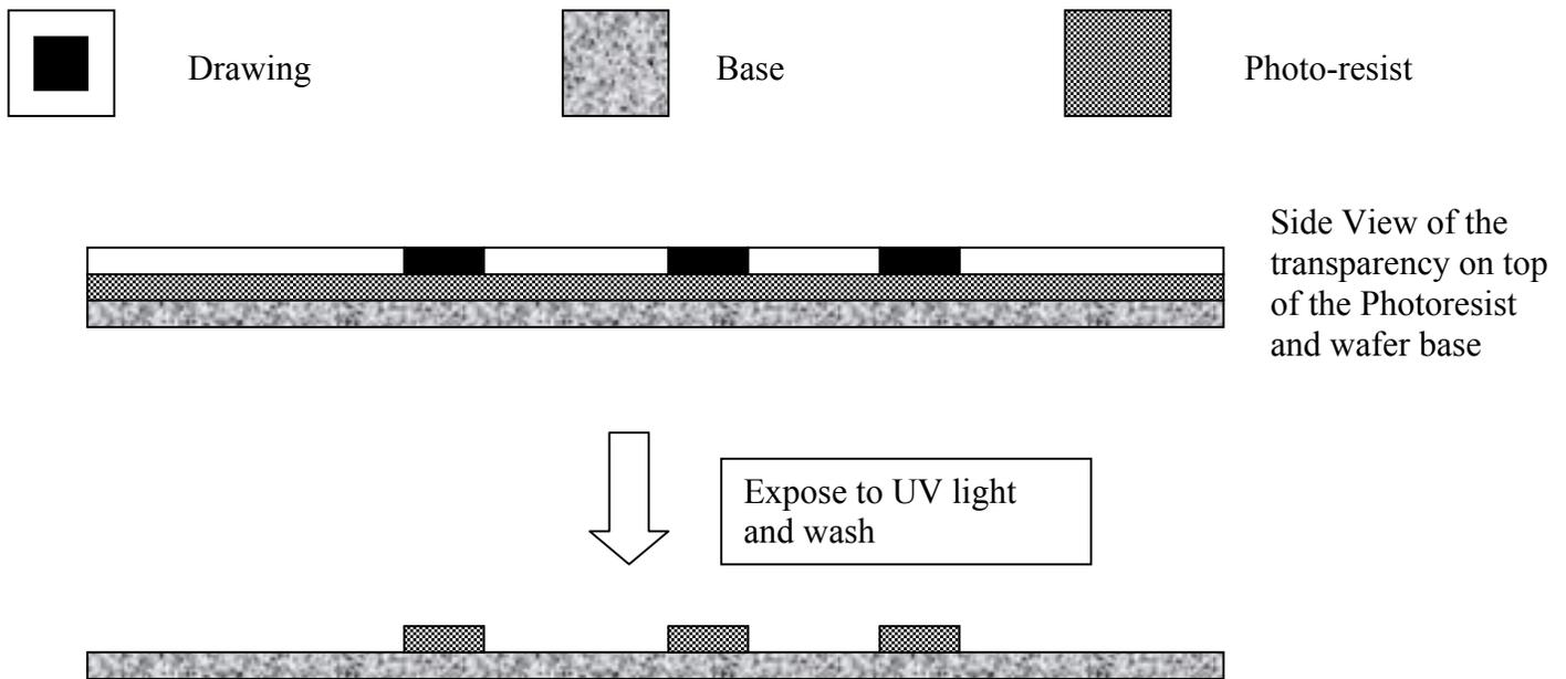
**Figure 3. Fabrication of the flow layer of a microfluidic chip.**
